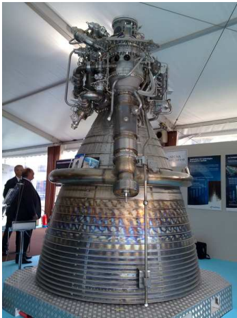
Ariane 5's Vulcain 2 engine liquid oxygen/liquid hydrogen
